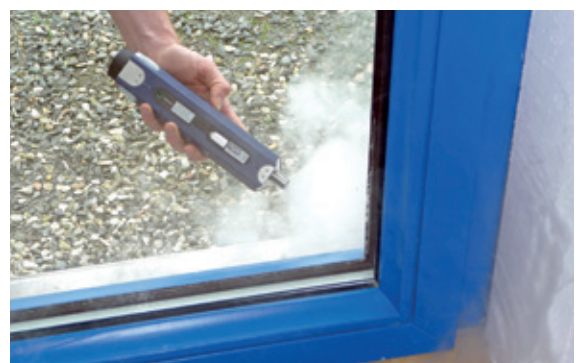
Leakage detection with the fog generator BlowerDoor HandFogger
