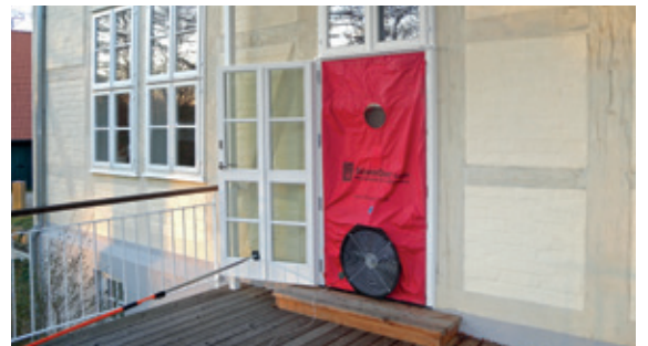
BlowerDoor measurement in the context of an energetic renovation
