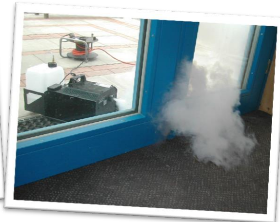
The HandFogger (630 g, 70 watts)
