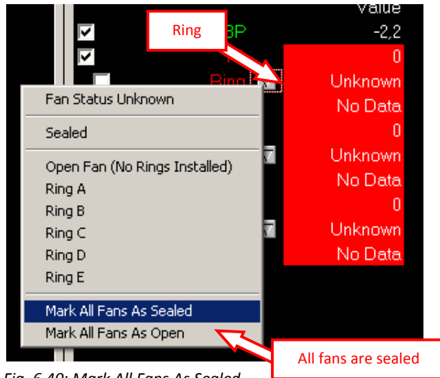
Fig. 6.40: Mark All Fans As Sealed
