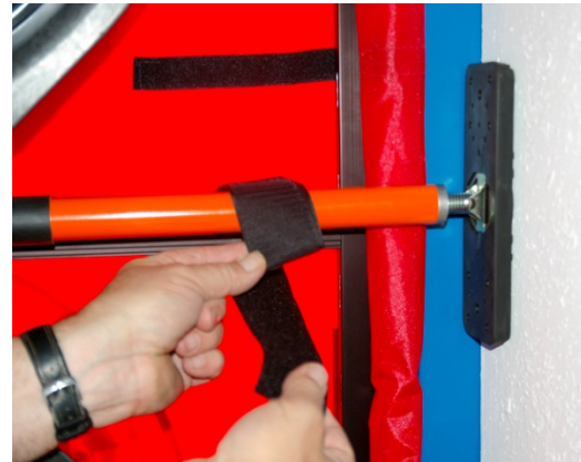
Fig. 4.5: Horizontal installation of the mounting strut
