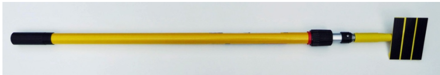
Fig. 3: Telescopic bar and handle with Velcro strips for Exhaust Fan Flow Meter.
