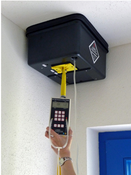
Fig. 7: The Exhaust Fan Flow Meter is placed directly over the exhaust fan grille and is pushed up against the wall or ceiling.
