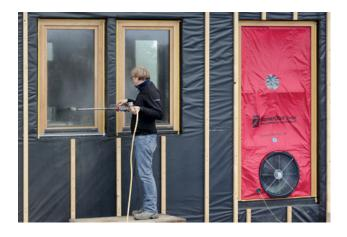
Ideally, the measurement should be conducted in combination with a Minneapolis BlowerDoor measuring system like BlowerDoor Standard or BlowerDoor Mini-Fan. Negative pressure tests are particularly suited to detect even small leakages. The tests can be further supported by using a thermal-imaging camera.
