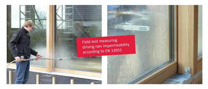
The SPRAY BAR helps you to detect larger leakages in curtain walls according to European Standard EN 13051 and can be used for testing the water tightness of windows, French doors, as well as external doors including all exterior components.
