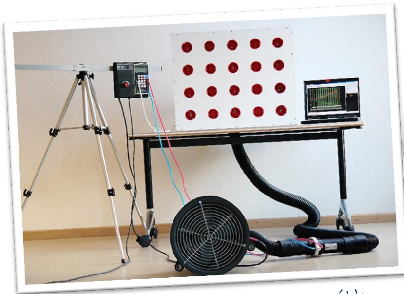
Testing building components with the Micro Leakage Meter (MLM)
